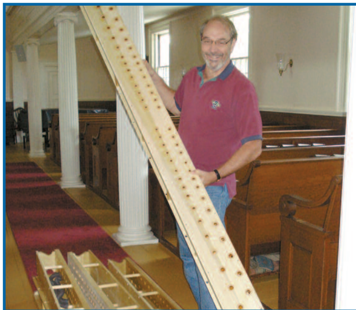
Tom Wilson with parts of the pipe chest.
